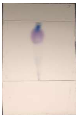
Figure 3. The thin-layer chromatogram obtained for ink sample 3, which was hydrolyzed in sodium hydroxide (NaOH) (photographed under daylight).
