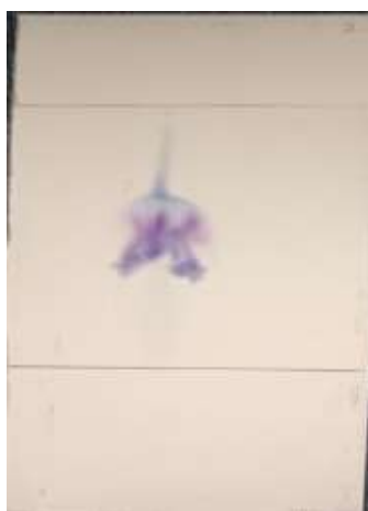
Figure 2. The thin-layer chromatogram obtained for ink sample 2 (acidic hydrolyzed condition), which was hydrolyzed in nitric acid (HNO 3 ) (photographed under daylight).
