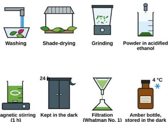
Figure 2 proves the extraction steps for each leaf and bracts from washing and shade-drying of the plant material to cold maceration, filtration and storage of the extract.
