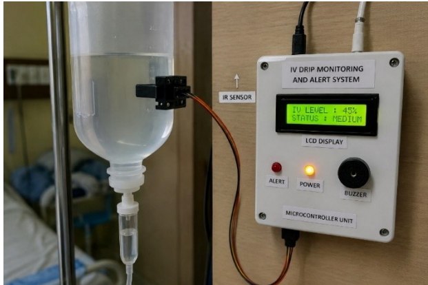
Figure 1: IV Drip Monitoring System
