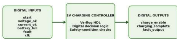
Figure 1: Block diagram of the EV charging controller.
