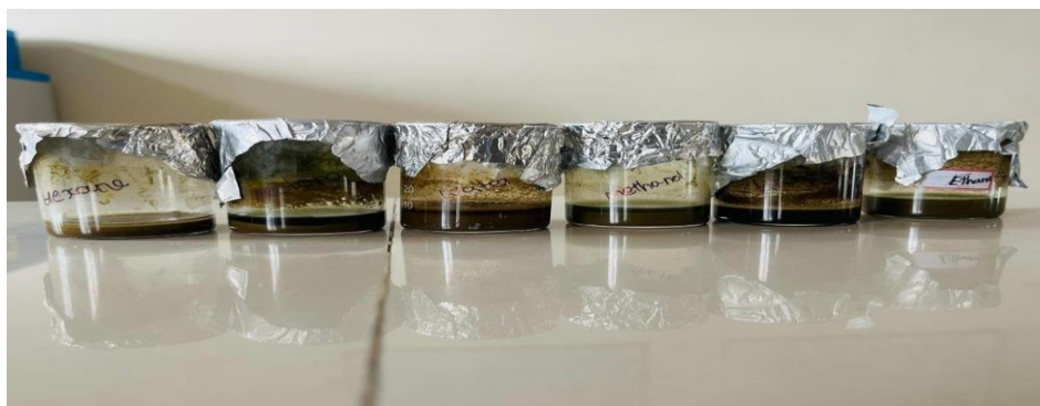
Fig. 6: Set-up used for determination of solvent extractive values (hexane, chloroform, methanol, ethanol)
