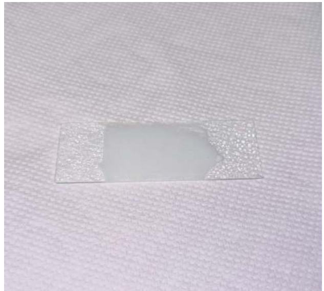
Figure B4: Chemical Coppertone Sunscreen Sample with Saline Solution Added
