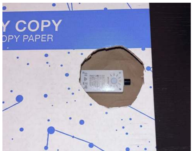
Figure B6: Bird's Eye View of UVA Sensor in the Cardboard Box
