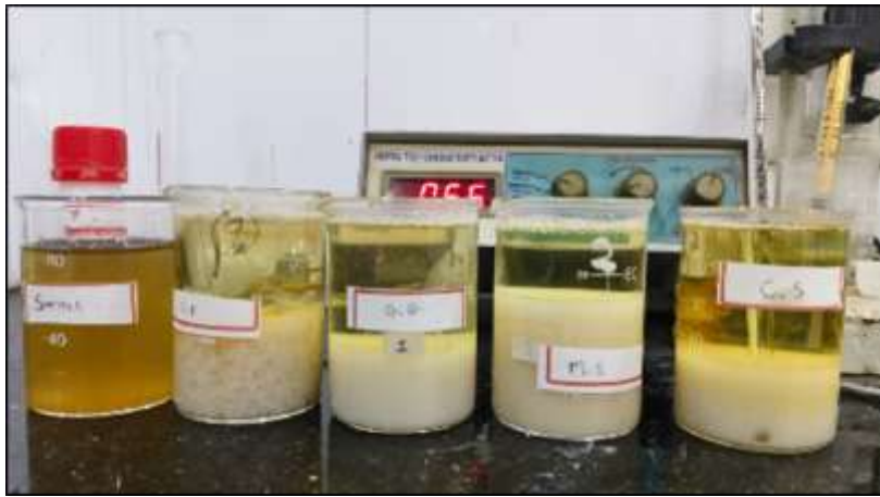
Figure 3: Jar Test Beakers of Treated Wastewater with Guar Gum and Different Coagulants After One Hour
