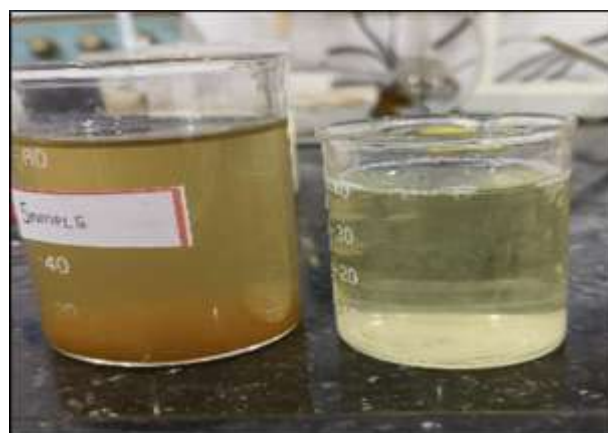
Figure: 2 Beakers Containing Sample (Raw ETP) and treated Sample with Guar Gum Solution
