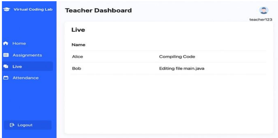
Fig. 5: Teacher Live Monitoring View. The WebSocket synchronization layer relays live code edits from students (e.g., Alice compiling, Bob editing) directly to the instructor's console.
